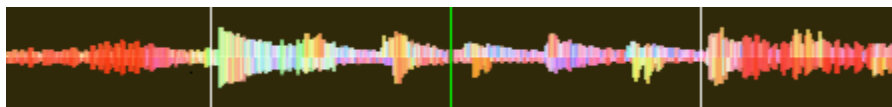
Figure1: A waveform at a good level. Note that the example waveforms in this section were made by adjusting the visual gain of the waveform display in Mixxx to illustrate the concepts. Adjusting the visual gain of the waveform display does not change the level of the audio.
